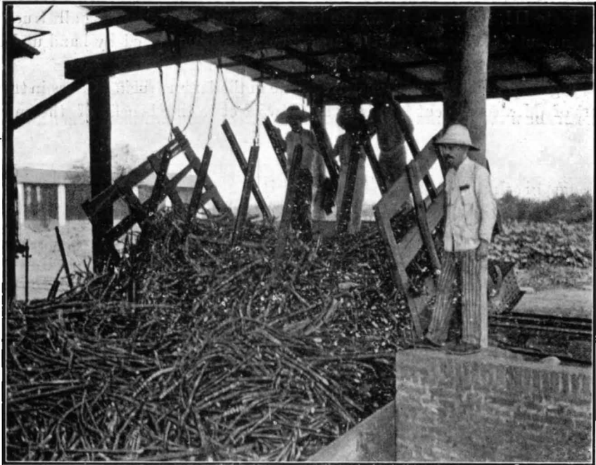
Fig. 4.—Bascule in a French Factory tipping a truck of cane into the carrier (wooden truck).
