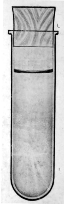
Fig. 8. Colour of the 10% solution of sugar produced by the alumina cream treatment.
