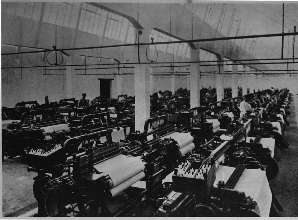
The newly-constructed Toyota Automatic Loom Shed of The Toyo Podar Cotton Mills Ltd., Bombay. (All transmission shafts are underground.)
