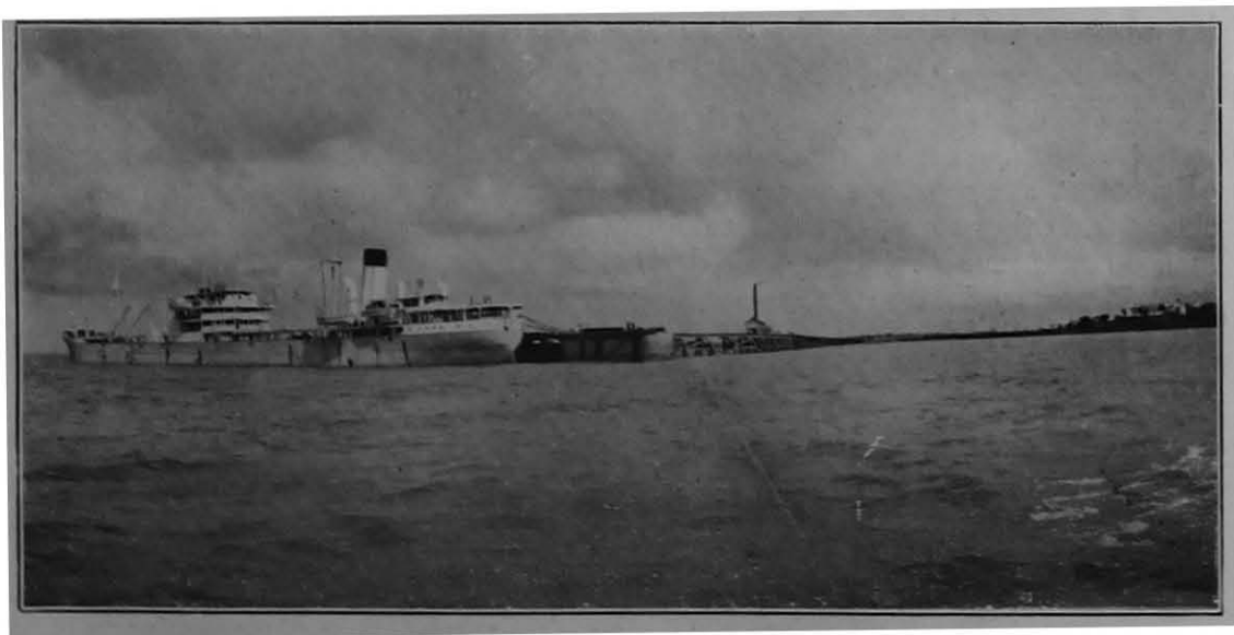
A tanker discharging bulk petrol at the bulk oil pier at Pis Pao.
