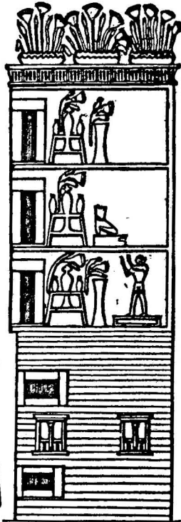
Fig. 81.—AN EGYPTIAN HOUSE, PARTLY IN SECTION.—See Page 130.
