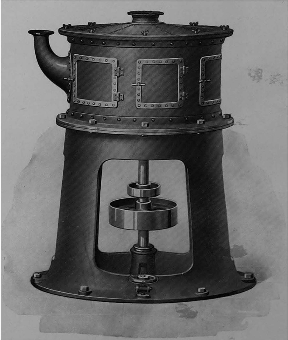
FIGURE 14. Self-Contained Pearling Cone. For whitening the shelled Rice.
