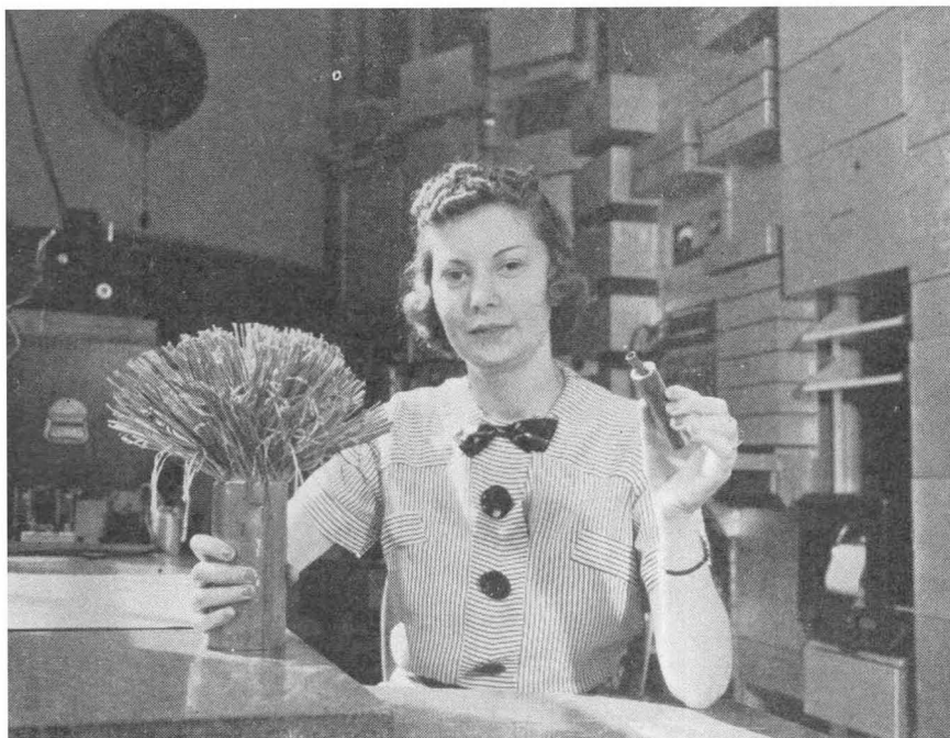
Figure 10. Today you talk over a wire; Tomorrow you'll see over one. On left is a section of cable, containing 600 wires, such as now is used for long-distance calls and network radio programs. At right is a section of the new "coaxial" cable, over which you can "see" by television as well as talk. It is only one-ninth as large as the other and contains two flexible copper tubes, with a thick wire inside of each. Waves like those of radio will carry 240 conversations at once through this cable, each at a different frequency. Other waves will carry television pictures over the same channel. Copyright National Geographic Society.
