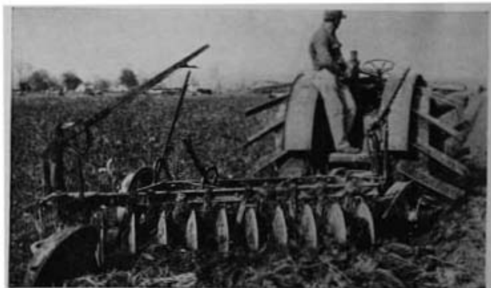
A heavy duty tractor may replace a dozen mule team and handle a six foot disc plow cutting five inches deep, thus speeding up soil preparation.
