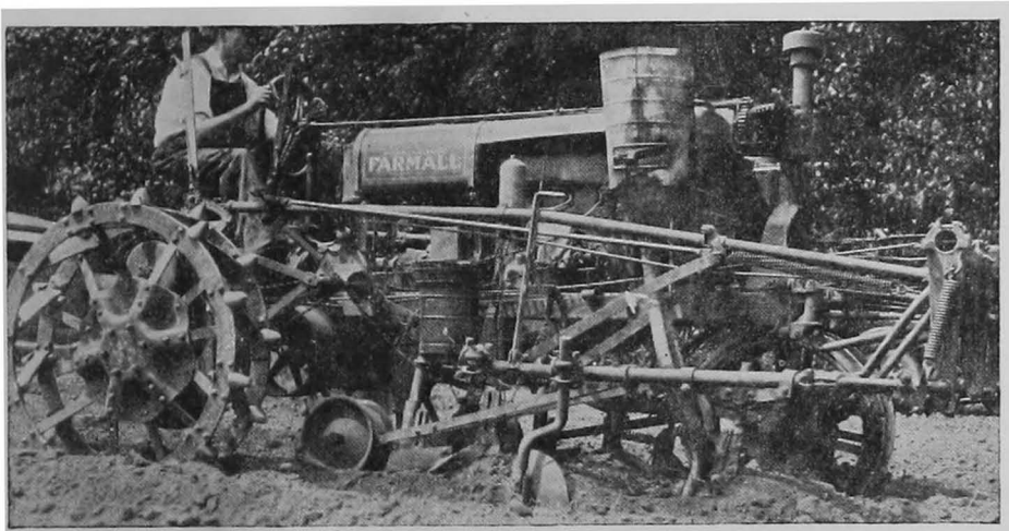
This outfit is putting in fertilizer, bedding and planting two rows of cotton at one operation.
