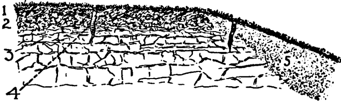
FIG. 2.—Formation of Soil. 1, thin layer of mould; 2, layer of shattered rock, partly derived from underlying rock; 3, the underlying compact rock on clay bed; 4, pockets, often seen in chalk, showing where trees have stood and caused borings through long-continued root action; 5, gravel bed resting on flanks of a slope.
