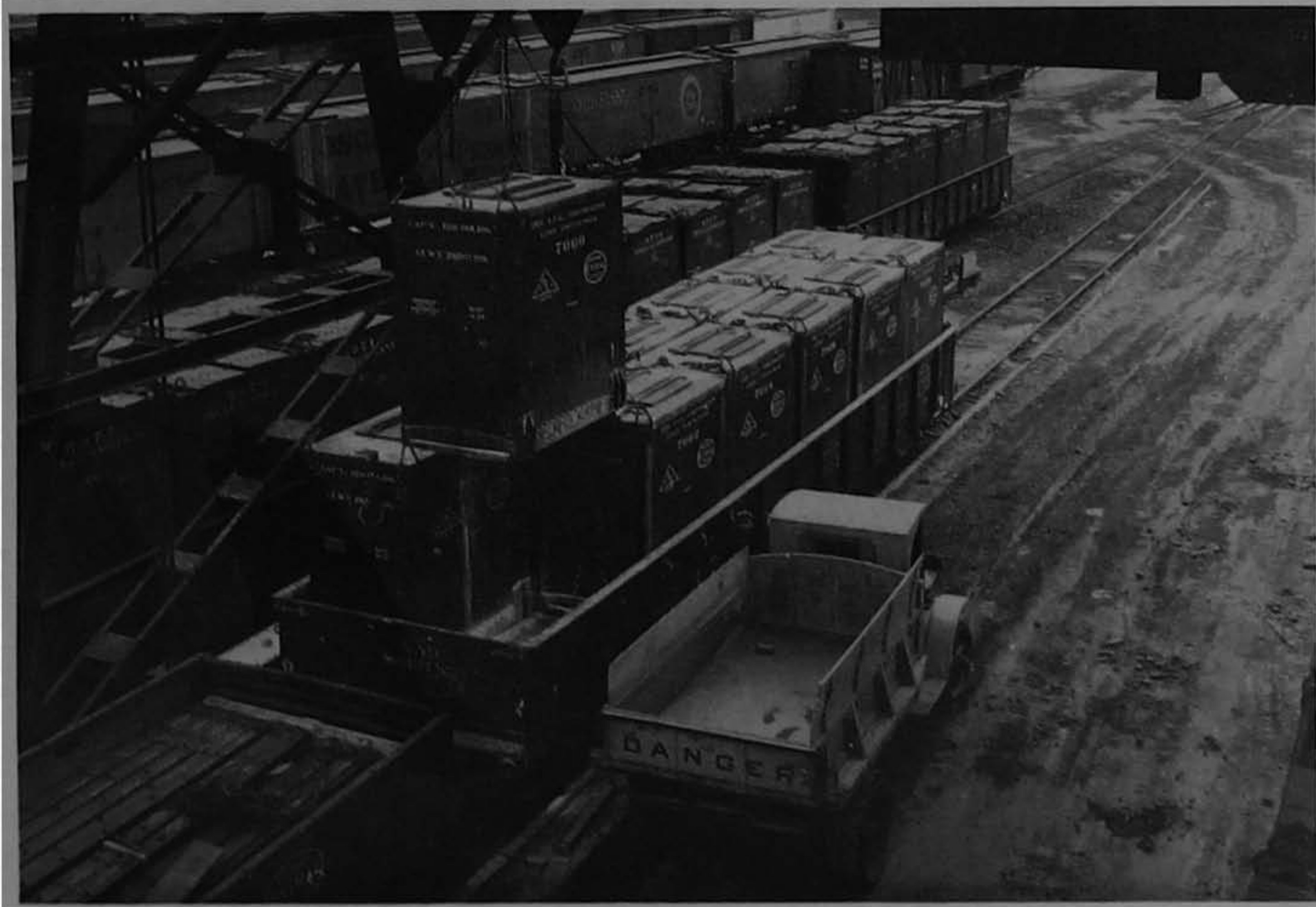
FIGURE 2 Transfer of lime containers (Brick containers have same dimensions.)
