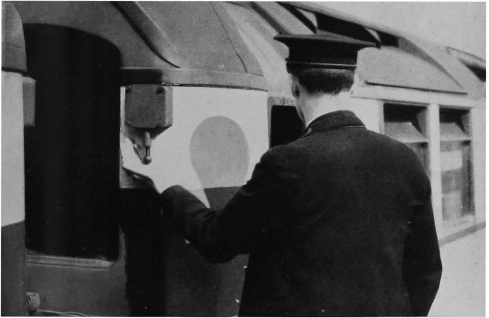
Fig. 71. The plunger can be operated by the platform staff for the purpose of closing air-controlled doors in the front part of the train.
