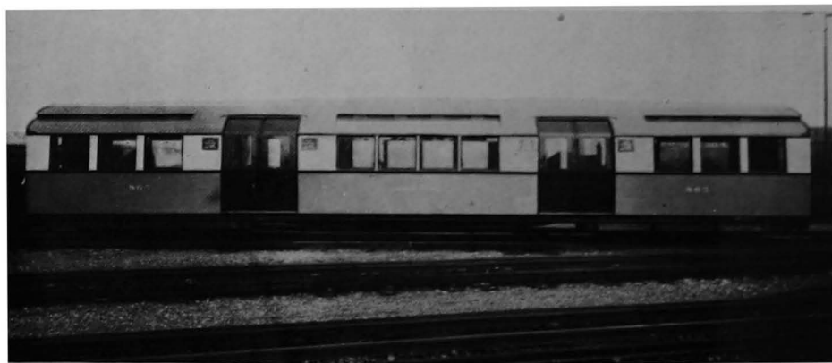
Fig. 66. A car with the new type of air-controlled doors.
