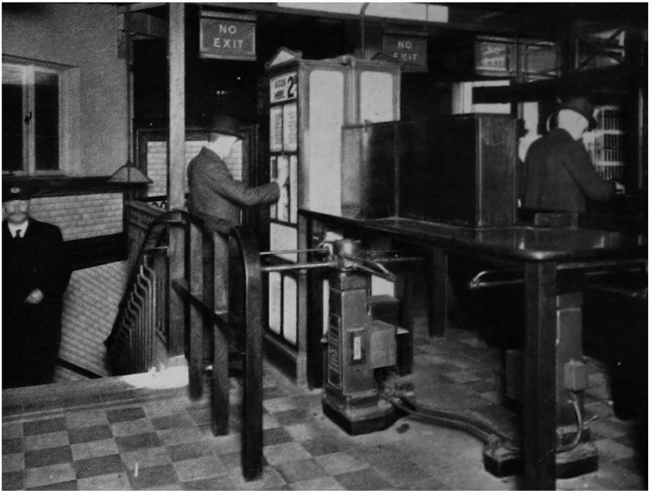
Fig. 103. Automatic machine used in conjunction with passimeter equipment.
