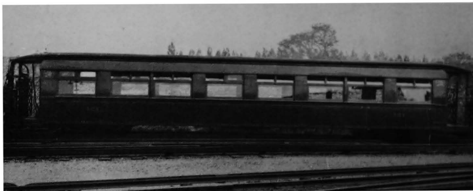
Fig. 65. A car equipped with the end doors that have now been superseded.
