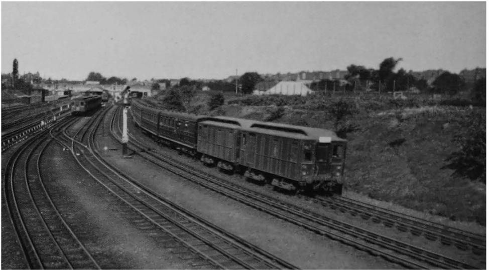
Fig. 145. An Ealing—Southend train being hauled over the District Railway by an electric locomotive.
