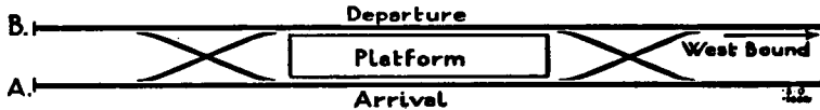
Fig. 26. Liverpool Street, Central London Railway, an example of a terminal with a cross-over at each end of an island platform.
