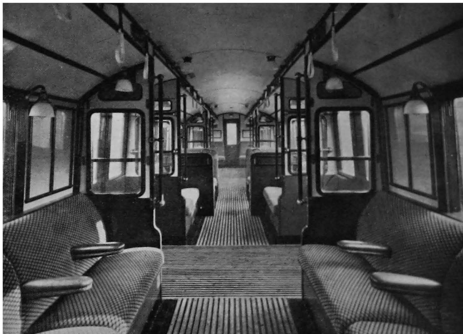
Fig. 100. Interior of the new-type City and South London Railway car.
