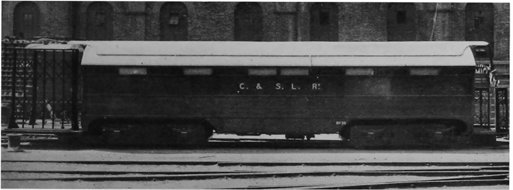
Fig. 85. Exterior view of one of the original City and South London Railway cars, in service in 1890.
