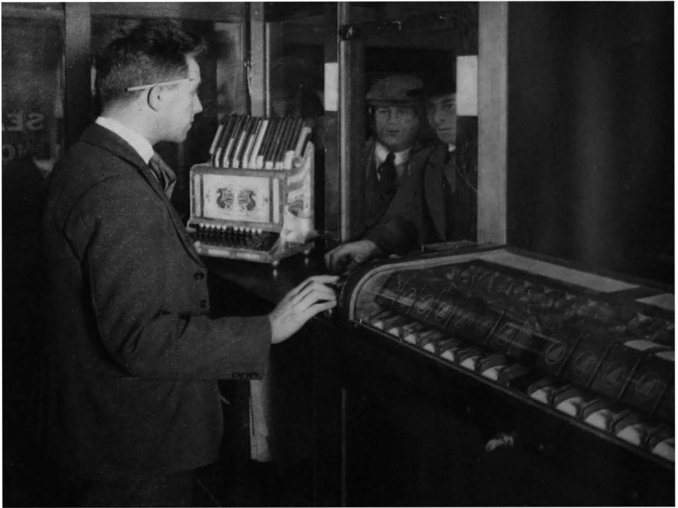
Fig. 107. Interior of a passimeter booth equipped with an automatic ticket-printing and issuing machine and (on left) a change-giving machine.
