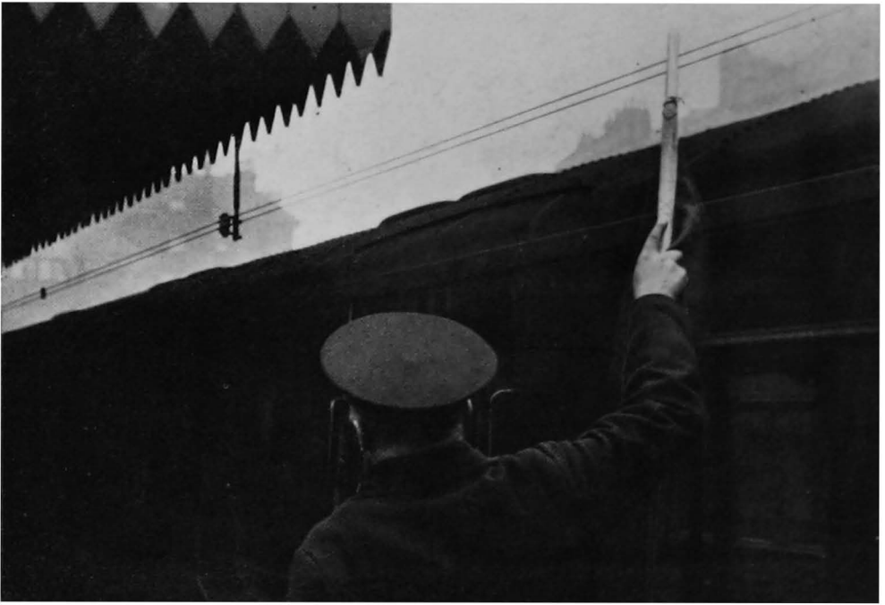
Fig. 123. A guard giving the 'right-away' by placing the metal handle of his flag against two wires, suspended above the platform, which causes an electric bell to ring near the motorman's cab.
