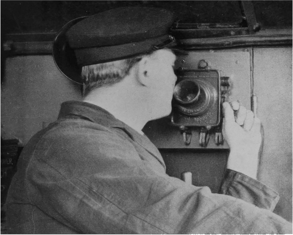
Fig. 69. A driver telephoning to the guard on one of the new trains; notice the loud-speaker just behind the driver's head and in line with his left ear.
