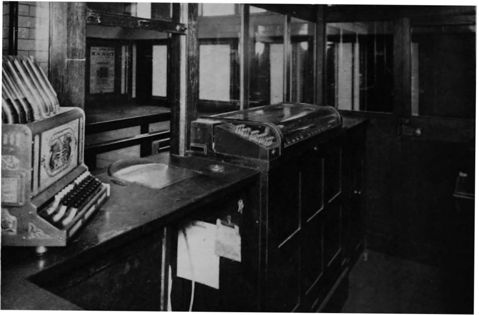
Fig. 110. Another interior view of a passimeter booth, showing (on left) the booking-clerk's change-giving machine, the new type of brass change-plate, and (on right) a ticket-printing and issuing machine.
