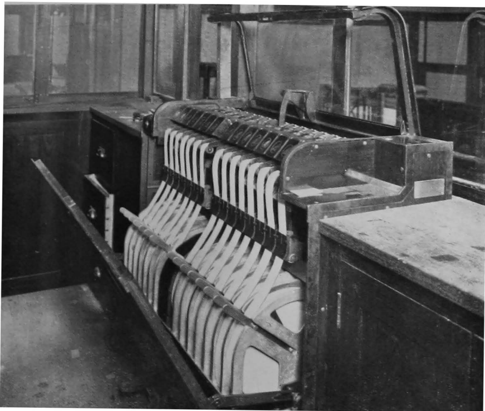
Fig. 108. Interior of an automatic ticket-printing and issuing machine.
