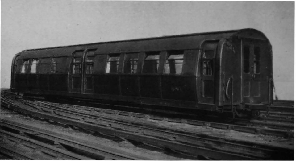
Fig. 95. A modern London Electric Railway car, with pneumatically operated doors.
