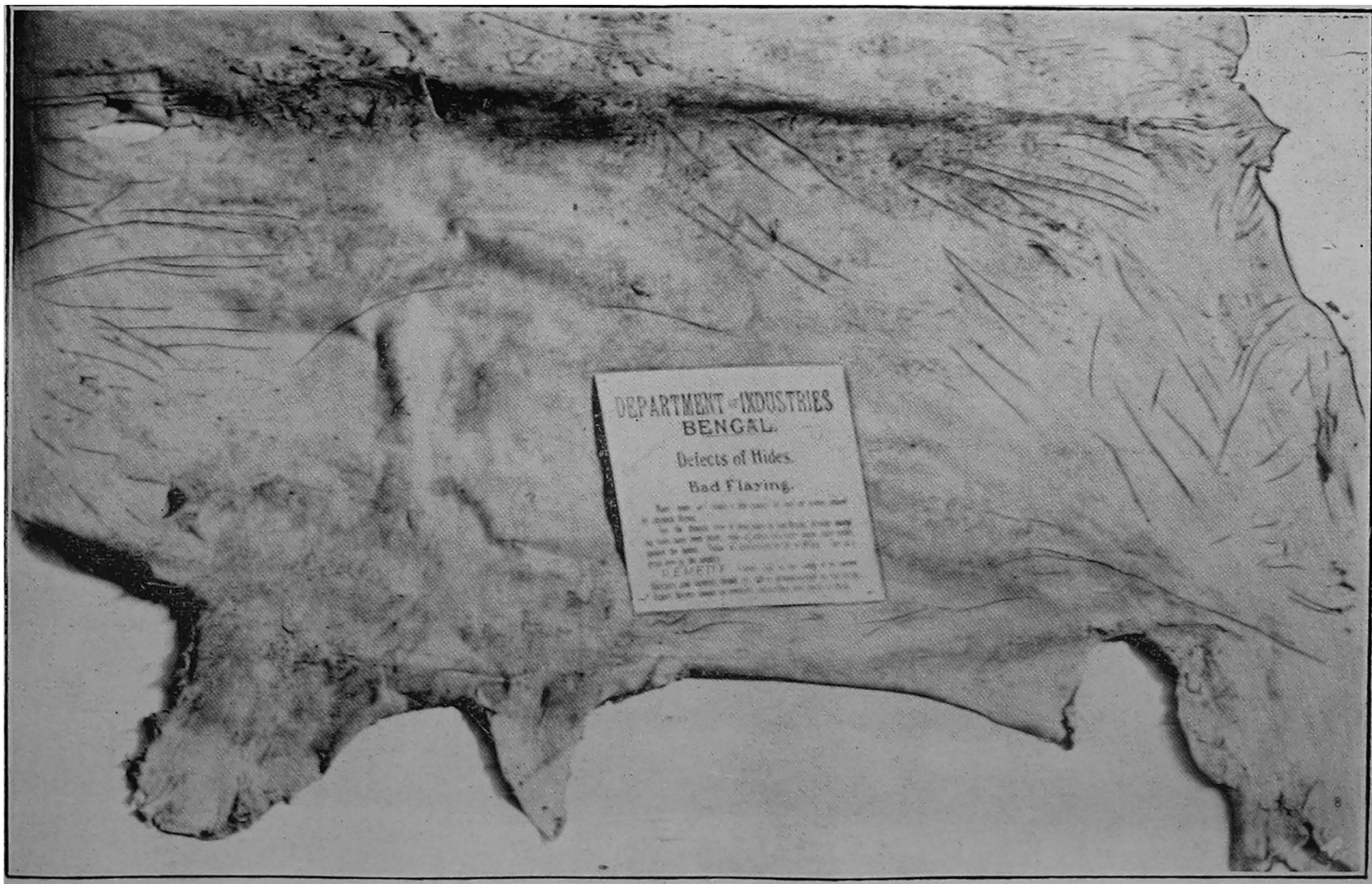
No. R-14.—Bad flaying.
