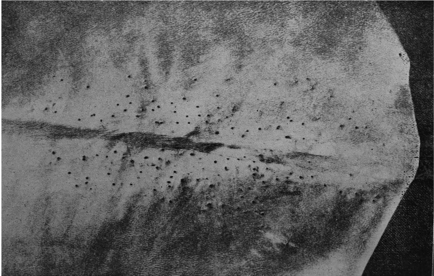
Portion of "grubby" hide of a cow after being tanned. Practically ruined by holes made by cattle grubs in the most valuable part.
