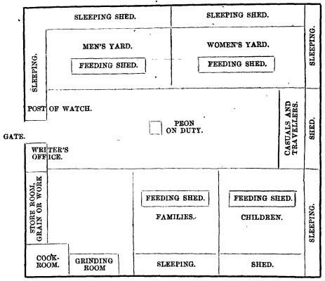
The above sketch may serve as a suggestion as to the way in which a poor-house should be laid out and arranged.
