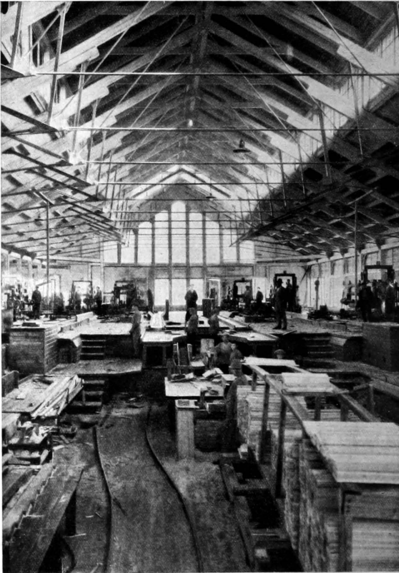
Interior of a modern sawmill with three-level floor. (Skoghall Sawmills, Uddeholms A.-B.)
