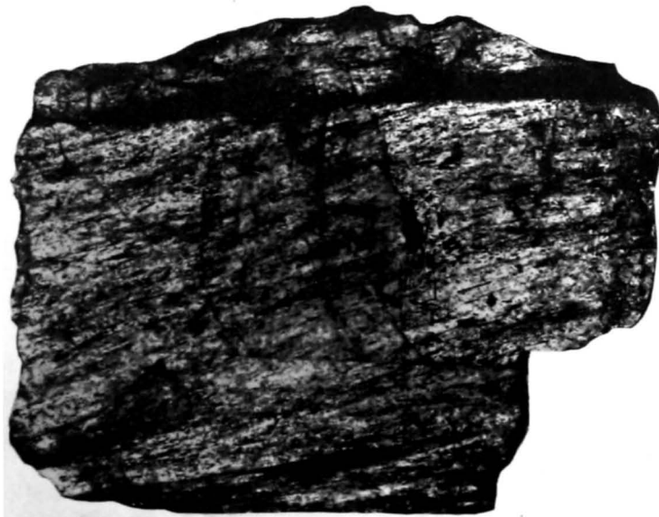
FIG. 2. PORTION OF CRYSTAL OF NATURALLY RECRYSTALLIZED BITUMINOUS SALT, Showing schistose arrangement of the bituminous matter through the crystal. Photographed by transmitted light ( \times 2 ).
