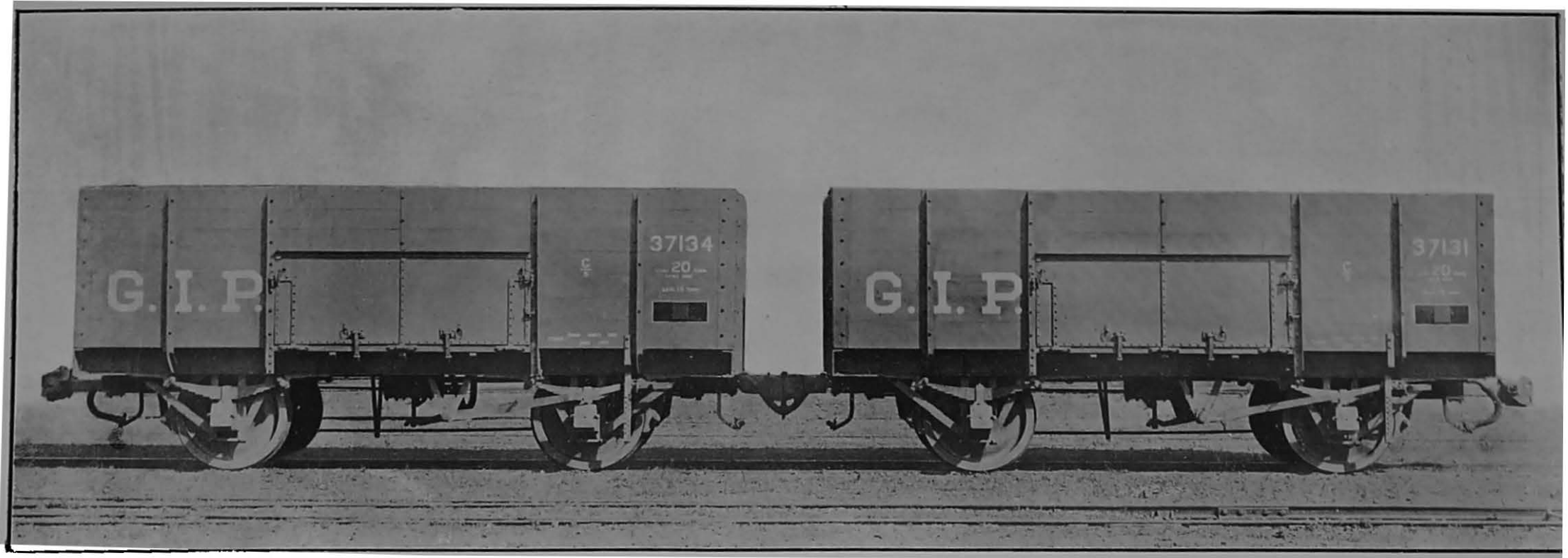
Rebuilt Wagons on the Great Indian Peninsula Railway, coupled with "Simplex" Automatic Central Couplers.
