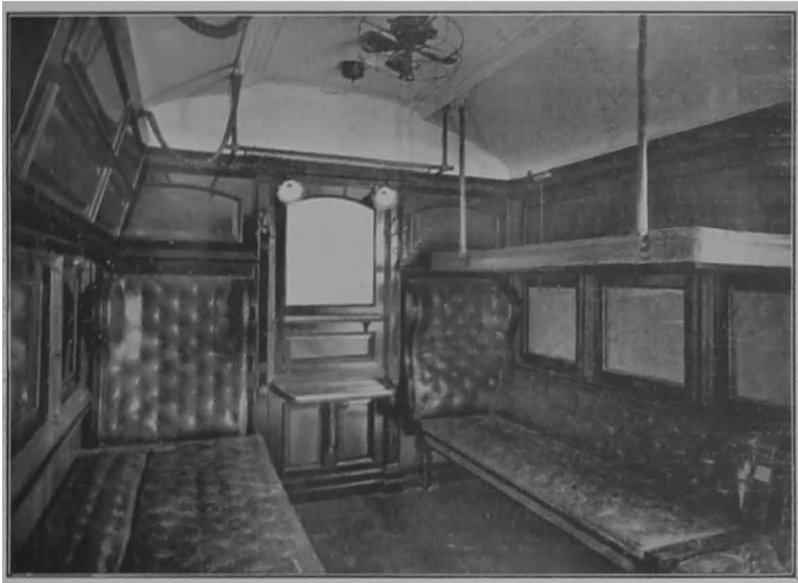
Interior of 1st-Class Compartment showing Folding Berth.—East Indian Railway.
