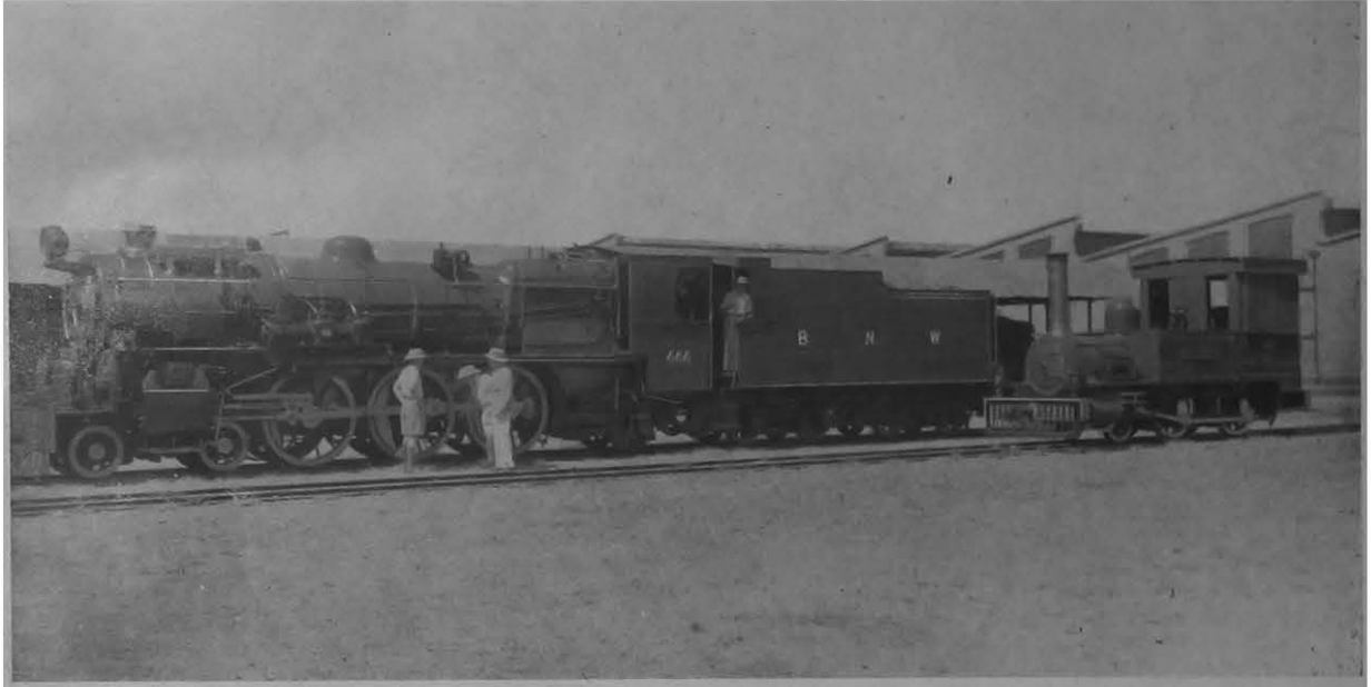
Engine No. 1 Lord Lawrence with a tractive effort of 3,857 lbs. put on line in 1874 and Engine No. 444 fitted with Caprotti valve gear, A.C. F. I. water heater and a tractive effort of over 16,000 lbs. put on line in 1938.
