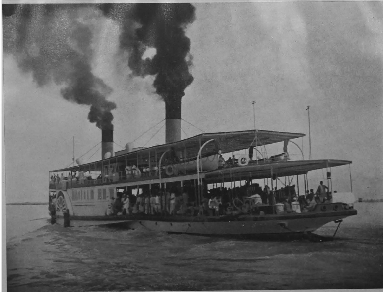
Ferry Passenger steamer 'Samastipur' crossing the Ganges from Mokameh to Semariah Ghat (500 tons with engines of 1,050 indicated horse power : put into service in 1929).
