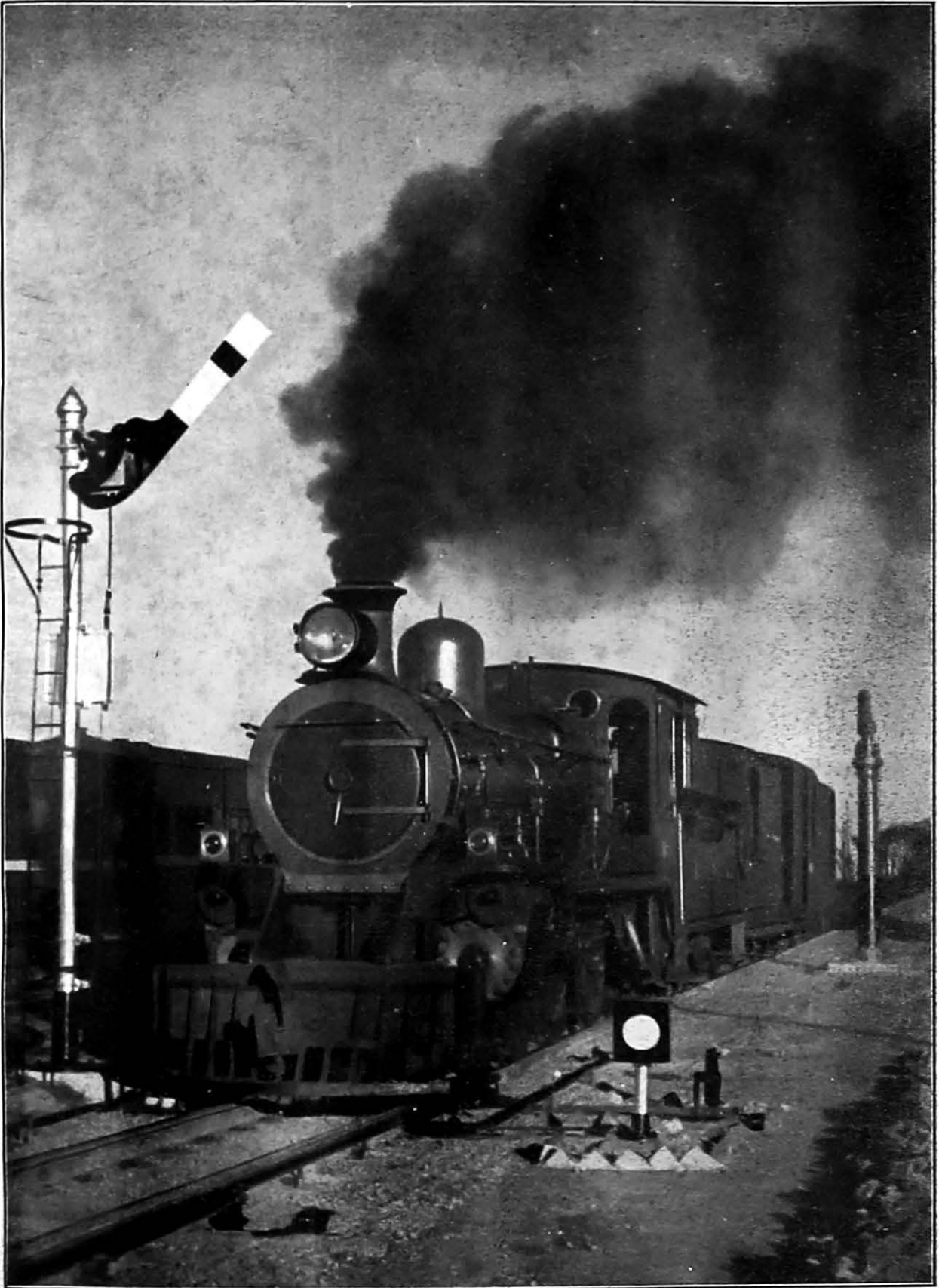
A goods train starting from Bhairab Bazar station under " Caution Aspect " : illustrating the use of double-wire 3-aspect signalling.
