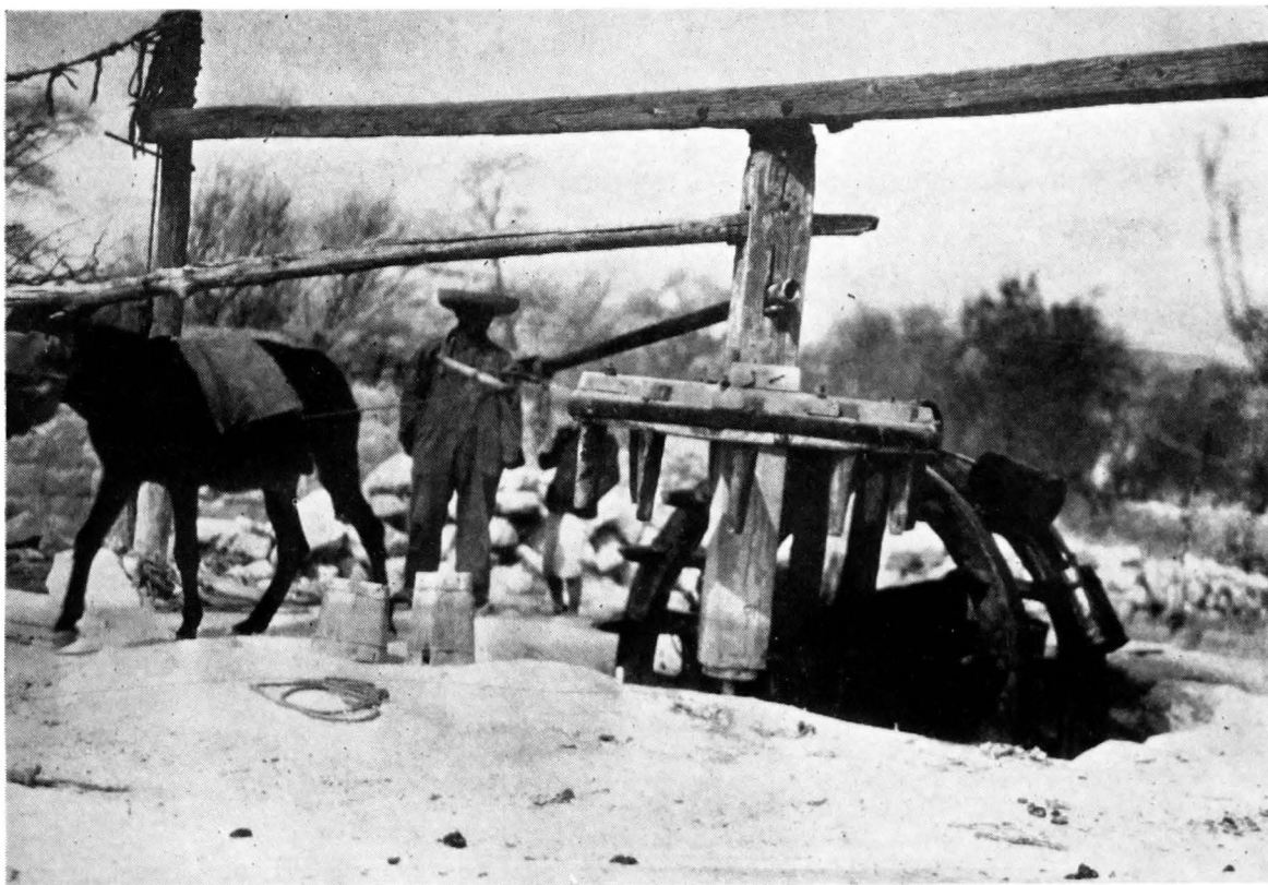
A Method Used by Many Mexican Villages in Their City Water Department. Notice the Gear Wheel Made From Wood Pegs. The Author Visited a Small Rural Farm and Found a Similar "Pump" Used for Irrigation Where Man Furnished the Power Instead of Burro.
